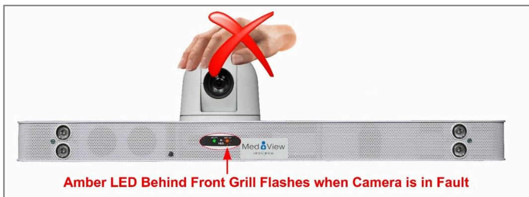
Figure 22 – Camera Fault Condition Indicator
