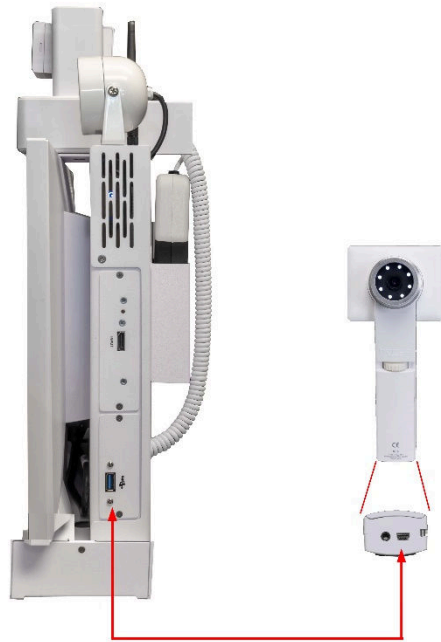
Figure 3. Horus Scope – CLINiC Connectivity Diagram
