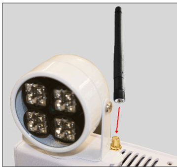
Figure 11 - Installing W-Fi Antennas
