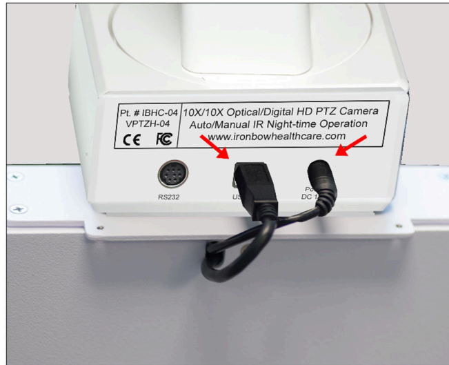
Figure 5 - Connecting the two camera cables
