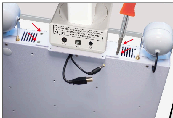
Figure 4 - Attaching Mounting Plate to System Chassis
