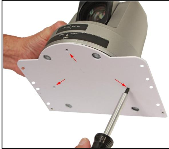
5. Gently place the camera assembly on top of the support bracket, ensuring the locating holes on the base plate line up with the holes on the mounting plate.
