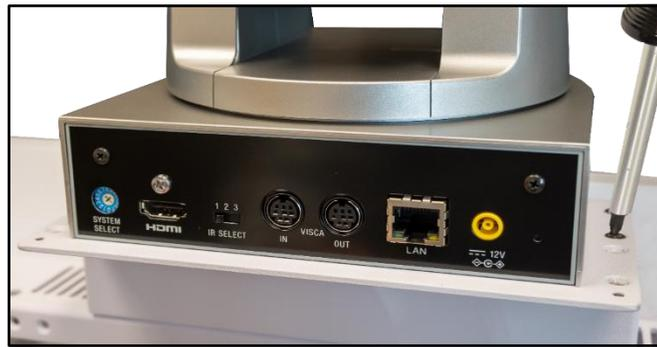
6. There are two sets of holes available for attaching the mounting plate to the system (see Figure 3 above). The selection of which holes allows the camera to overhang more at the front or the rear, depending upon how the system is to be installed:
