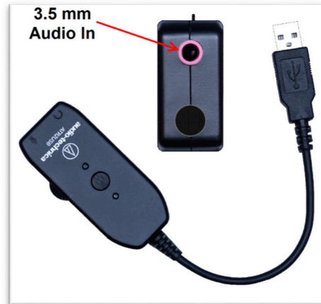
Figure 9 - 3.5 mm audio adapter
